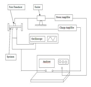
Figure 4 : Schematic Diagram of Experimental Setup
