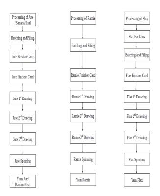
Fig.2. Processing Steps of Natural Fiber
